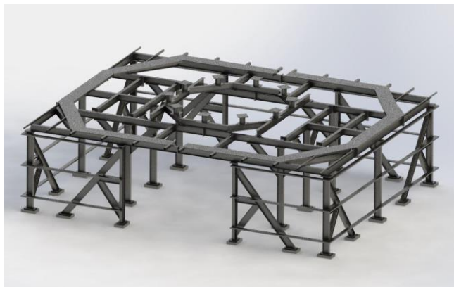
Figure 4: Steel structure of the shelter and control cubicle inside the shelter.
